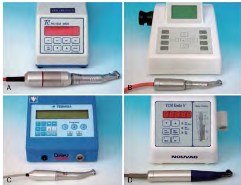
FIG. 6-30 Examples of motors used with rotary nickel-titanium endodontic instruments. A, First-generation motor without torque control. B, Fully electronically controlled second-generation motor with sensitive torque limiter. C, Frequently used simple torque-controlled motor. D, Newer-generation motor with built-in apex locator and torque control.
