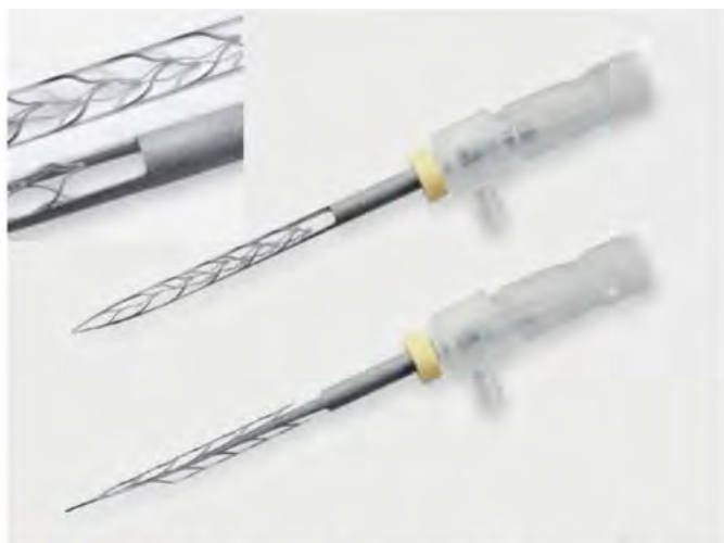
FIG. 6-26 The SAF instrument. The instrument is made as a hollow, thin NiTi lattice cylinder that is compressed when inserted into the root canal and adapts to the canal's cross section. It is attached to a vibrating handpiece. Continuous irrigation is applied through a special hub on the side of its shank. Inset shows the abrasive surface of the instrument. (Courtesy ReDent-Nova, Ra'anana, Israel.)
